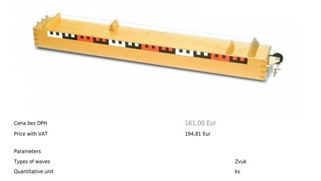
The Demonstration Monochord investigates the relationship between the pitch of a sound and the length of the string. Also investigate overtones formed by harmonic waves with intermediate nodes and the dependence of the pitch on string tension.
